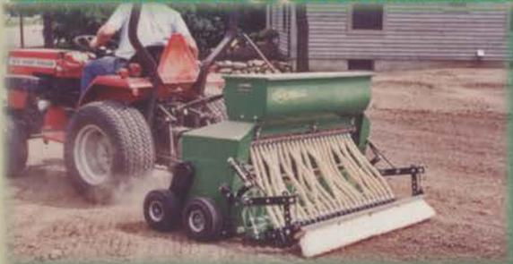
Put the Gandy Dethatcher Overseeder to work in your business. You'll be amazed at its performance. It is unmatched for quality, precision and economy. The unit is 48 inches wide with 24 blades to create slits on 2-inch centers. The overseeder has a stainless steel hopper bottom and slides and holds 100-125 lbs of seed.
