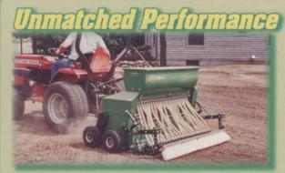
Put the Gandy Dethatcher Overseeder to work in your business. You'll be amazed at its performance. It is unmatched for quality, precision and economy. The unit is 48 inches wide with 24 blades to create slits on 2-inch centers. The overseeder has a stainless steel hopper bottom and slides and holds 100-125 lbs of seed.
