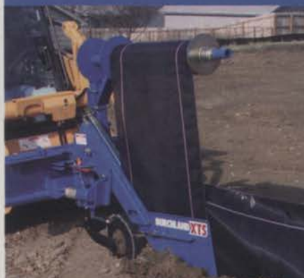
XTS Silt Fence Installer
