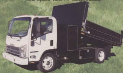
Isuzu NPR HD with 12' Dump Body 325 HP Gas Engine, Automatic Transmission, 14,500 lb. GVWR, 19.5 Tires, AM/FM CD Player, A/C, P/S, Power Windows & Locks, Tilt Wheel, Tow Package & Brake Control, (Other Options And GVW Ratings Available)
