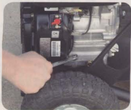
Run a tight ship: Check the engine's bolts to keep it from bouncing around.
