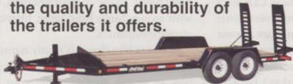
The Specialty Transport series of trailers offers great flexibility with I-beam construction and 82" between fenders with the deck made from 2" nominal bolted oak.
