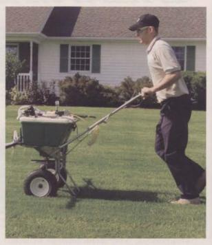
On his typical 9,000-square-foot jobs, Eric Zars uses the Spreader-Mate, a 9-gallon unit that he drops into a spreader, turning it into a walk-behind sprayer. Photo: Gregson-Clark
