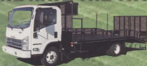
Isuzu NPR with 19' Dovetail Landscaper Body 325 HP Gas or 205 HP Diesel Engine, Automatic Transmission, 12,000 lb. or 14,500 lb. GVWR, Exhaust Brake (Diesel Only), AM/FM CD Player, A/C, P/S, Power Windows & Locks, Tilt Wheel, (Other Options And GVW Ratings Available)
