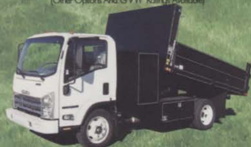
Isuzu NPR HD with 12' Dump Body 325 HP Gas Engine, Automatic Transmission, 14,500 lb. GVWR, 19.5 Tires, AM/FM CD Player, A/C, P/S, Power Windows & Locks, Tilt Wheel, Tow Package & Brake Control, (Other Options And GVW Ratings Available)
