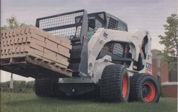
**Unleash a better way.** The A300's four steerable axles help minimize turf damage, tire marks on concrete and asphalt, and tire wear. That means less surface repair and cleanup as well as lower maintenance costs – and a better bottom line for you. Flip a switch and go from the smooth, rolling efficiency of an all-wheel steer to the agile maneuverability of a skid-steer. It's like having two machines in one.
