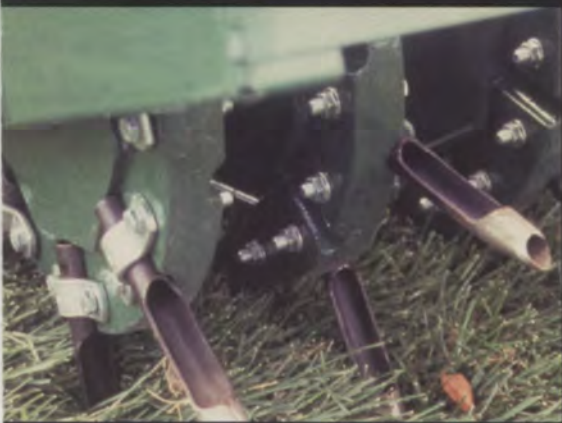
When shopping for an aerator, pay close attention to the tines. Look for ones that are going to remove a core, not just punch a hole.
