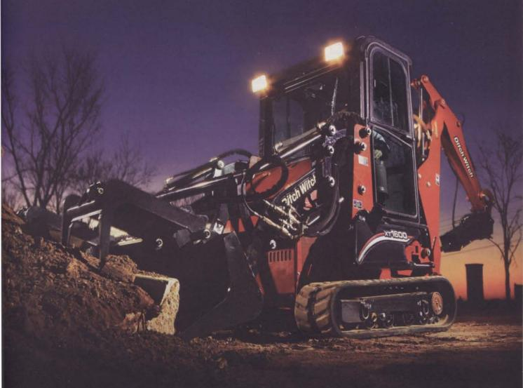
**The XT1600.** It's a backhoe loader, mini excavator, and skid steer all in one. Like its forerunner the XT850, it has a 260° excavator sweep that lets you dig at extraordinary angles in tight spots. And with 30 net hp to the tool carrier, it can run most full-size skid steer attachments. For details, call 800-654-6481 or visit ditchwitch.com.
