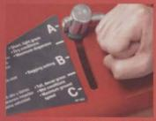
No-tools-needed adjustable baffle lets you quickly adjust cutting performance. As conditions change, Toros /-gauge TURBO FORCE® cutting deck can be quickly adjusted on the job to deliver an unbeatable quality of cut. To see the productivity-enhancing deck that professionals are raving about, contact your Toro Landscape Contractor Equipment dealer, or visit www.toro.com/zmaster.
