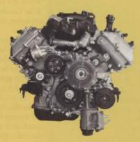
A metal duet. The big available V8's block is lightweight cast aluminum, but each cylinder bore is lined with a durable steel sleeve. So the engine efficiently expends energy hauling the weight of your payload, rather than itself
