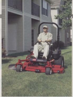
True to their name, zero-turning radius mowers can revolve 10 times before a standard mower can make a single revolution because of their unique pivoting action controlled by a pair of levers that enable the machine to turn, accelerate and break. Photo: Toro
