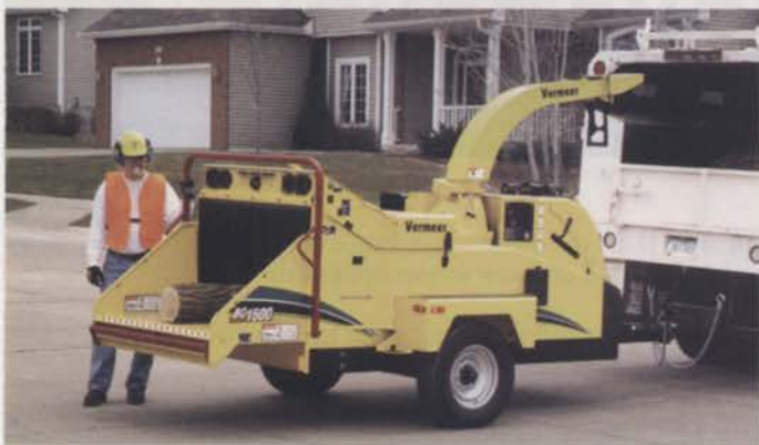
Job site chipping reduces the bulk of woody waste and allows the contractor to haul the material much more efficiently. Photo: Vermeer
