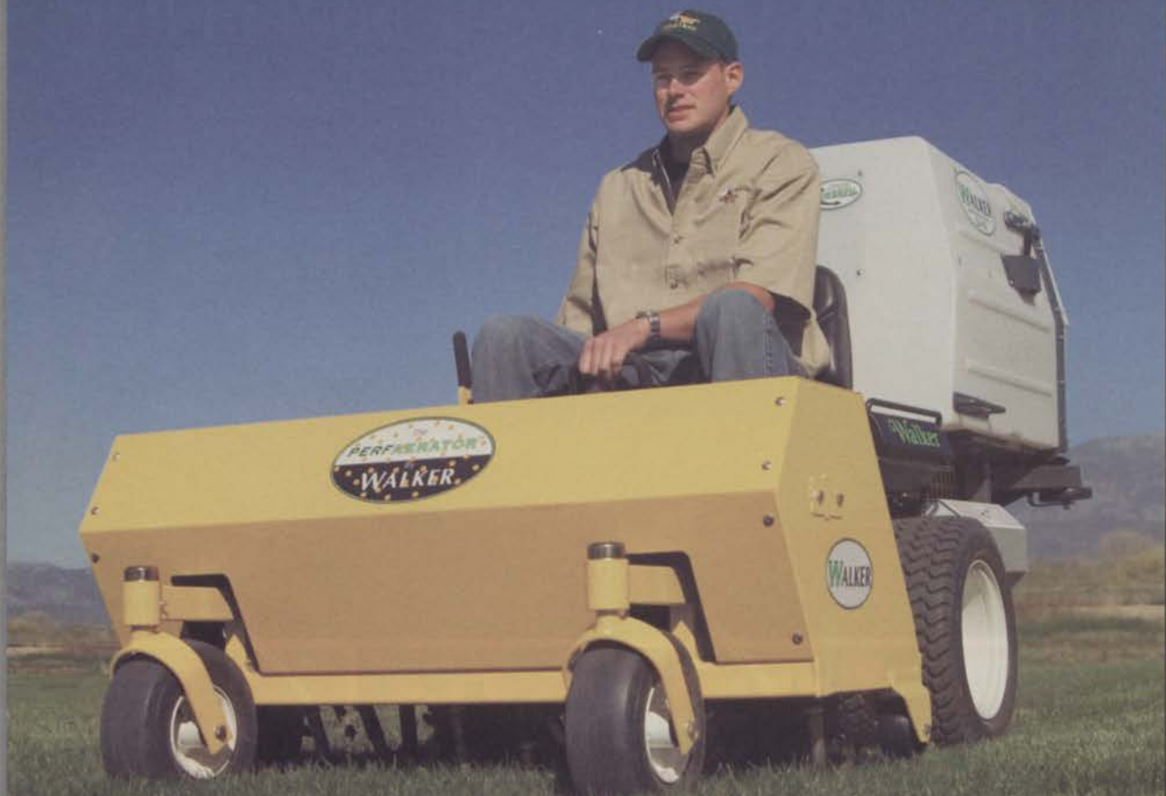
For contractors who only perform aerating on some jobs, an aerating mower attachment could be more productive than a stand-alone aerator. Photo: Walker
