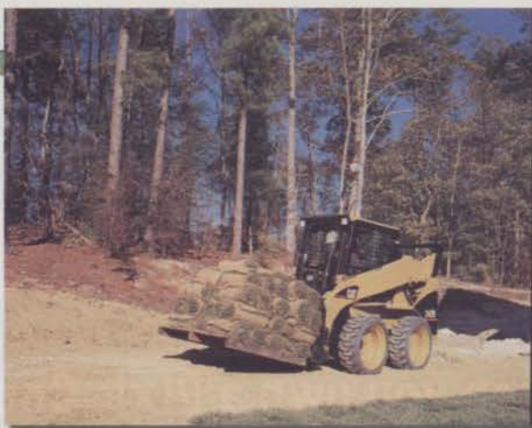
Skid-steers, which cost between $15,000 to more than $45,000, can be used for a host of tasks, including lifting and carrying materials, digging, grading and general ground preparation. Photo: Caterpillar
