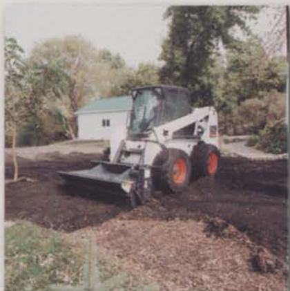
Skid-steers allow contractors to complete tasks in one day what may take a work crew a week to accomplish by hand. Photo: Bobcat
