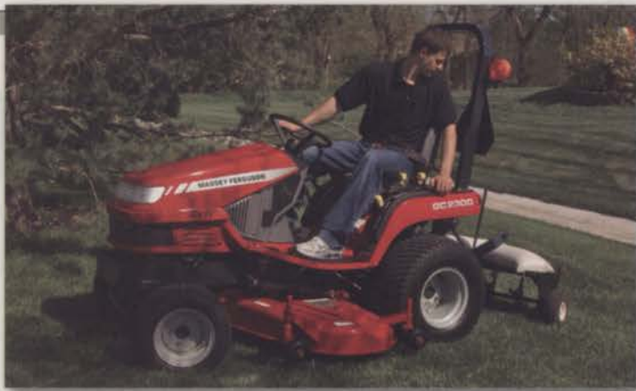
Some newer riding mowers are incorporating features that ease operator fatigue, such as cruise control and hydrostatic transmission where a foot pedal is used to switch gears. Photos: Massey Ferguson (above and pages 94, 95), Exmark (page 92)
