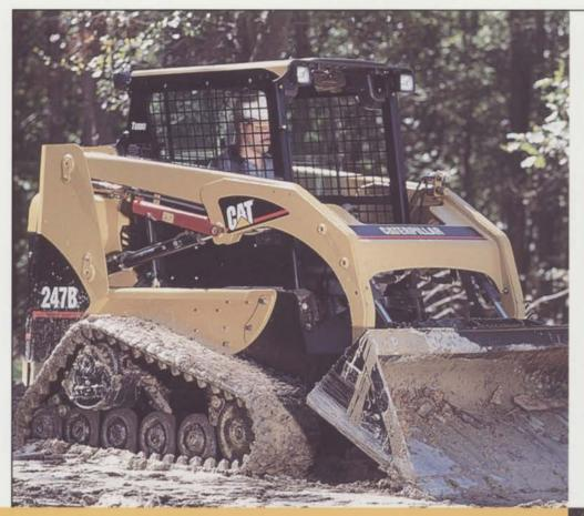
Cat" Multi Terrain Loaders feature a **suspended all-rubber undercarriage** for greater operator comfort and productivity. And they work in conditions and terrain that other machines can't match.
