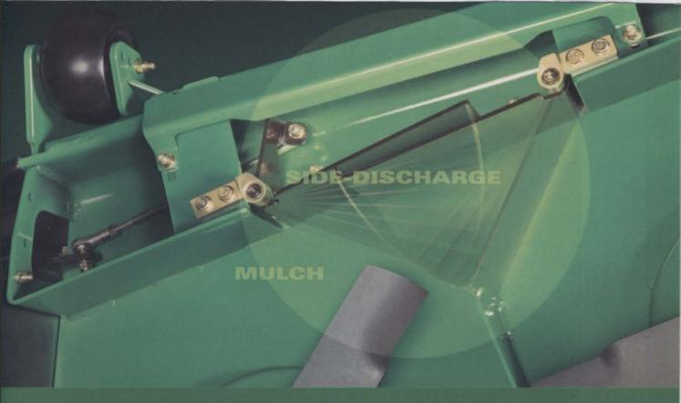
"In a matter of seconds, you can go from mulching to side-discharge. There's not another mower that can do that."
