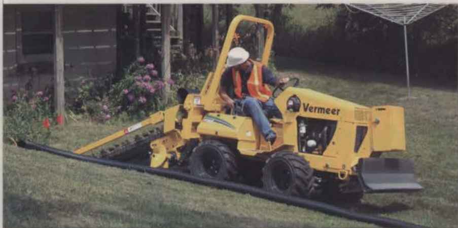
Ride-on trenchers offer more horsepower than walk-behind units. This translates into higher productivity, making them a good choice for large commercial jobs. Photo: Vermeer Mfg.
