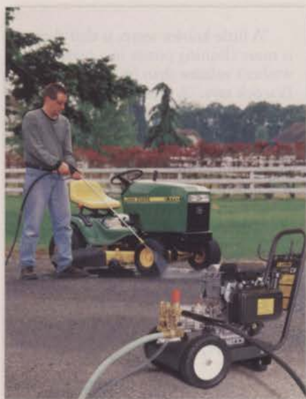
Pressure washers help contractors keep their equipment clean of grease and grime. Hot-water pressure washers are particularly well-suited for the task. Photo: Landa Pressure Washers
