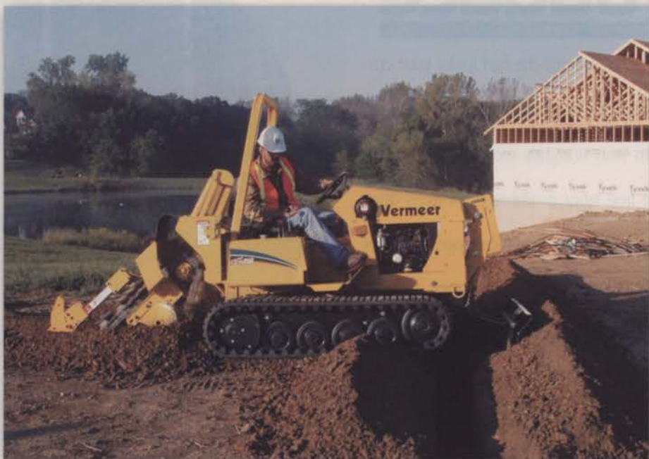
Digging by hand is rarely an attractive option on any job. That's why contractors are putting trenchers to work in a variety of tasks, including the installation of irrigation and landscape lighting systems. Photo: Vermeer Mfg.
