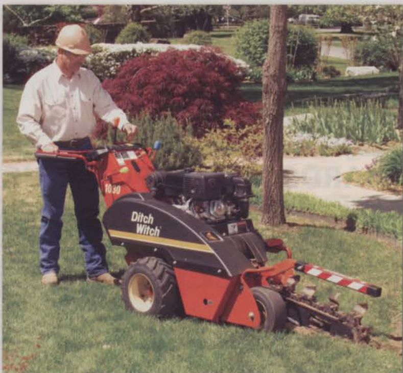
The compact size of walk-behind trenchers makes them easy to maneuver and transport. The machines are well-suited to residential jobs in which they have to fit through gates or into backyards. Photo: Ditch Witch
