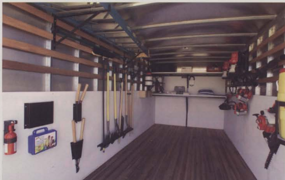
In an enclosed trailer or truck and trailer combination, a contractor should organize his tools and equipment. Organization is crucial because it can help crewmembers find tools more quickly, making them more productive. Keeping a tool in its place and away from constant abuse can also extend its life. Photo: Super Lawn Trucks
