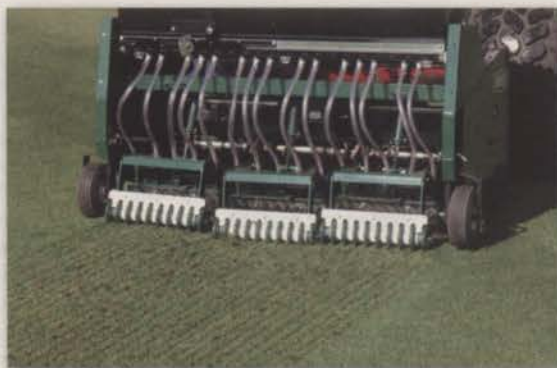
An overseeder creates slits in this turf to help achieve seed-to-soil contact. Photo: Turfco
