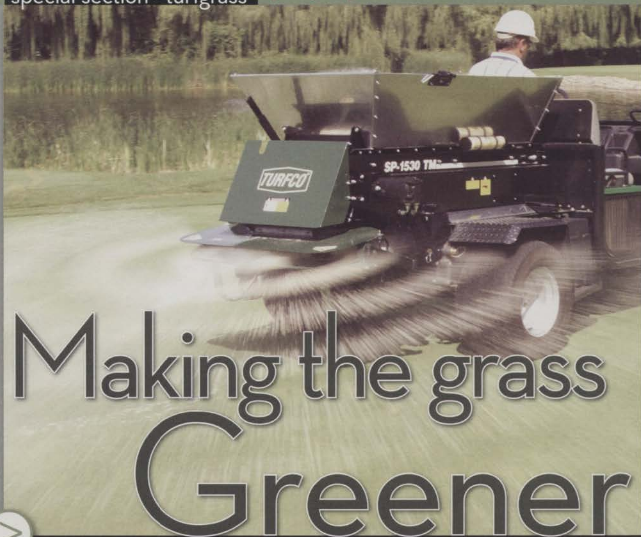
A spinner top dresser delivers seed to the turf. Photo: Turfco
