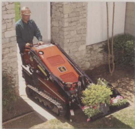
The mini skid-steer bucket attachment is, by far, the most popular because of its versatility. Photo: Ditch Witch
