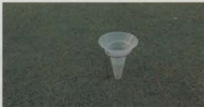
A catch can test can be used to measure the uniformity of an irrigation system. Photo: Brian Vinchesi
