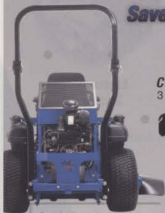
Oversized rear tires for excellent traction and overall handling, low soil compaction, and a smooth ride.
