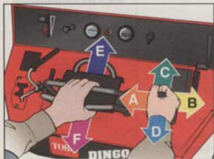
The Toro® Dingo® TX Control System operates with just three easy controls.
