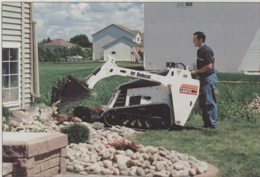
A bucket, like the one above, is one of the most popular compact utility loader attachments among landscape contractors. Choosing between walk-behind models and ride-on models is a choice as dependant on site specifications as it is personal preference. Photos: Bobcat (above), Toro (below)
