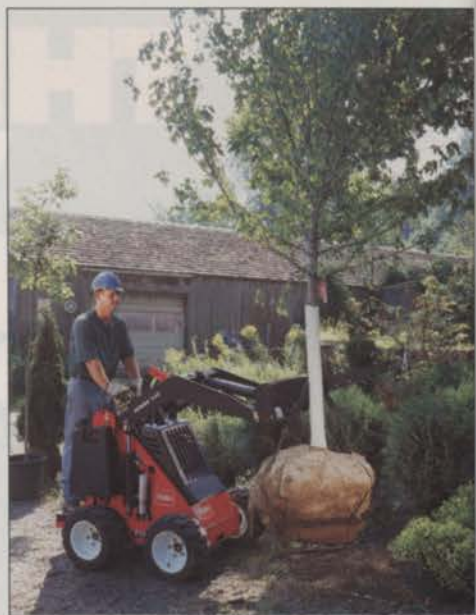
Manual labor used to be the only way to transplant a tree, but compact equipment can make the same job less strenuous and more efficient. Photo: Toro
