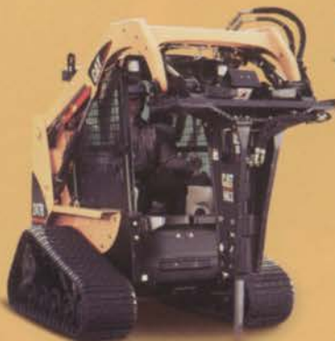
5 models of MTLs (57 to 78 hp) feature renowned Cat track technology.
