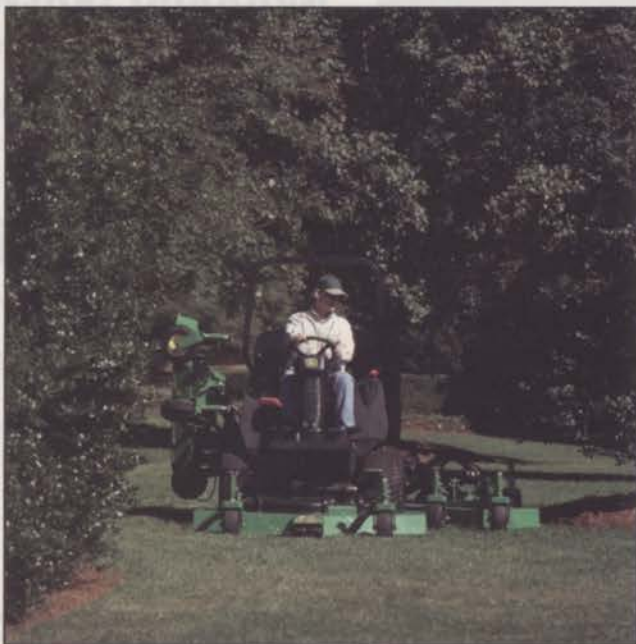
For tight areas, some wide-area mowers have spring-loaded side breakaway decks that will allow them to maneuver around trees or other obstacles and then spring back into place. Photo: John Deere
