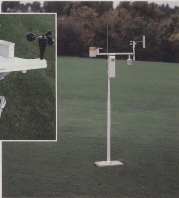
Weather stations gauge soil moisture and evaporation rates. In conjunction with an irrigation controller, the two create a data-driven irrigation program that can save contractors money. Photos: Campbell Scientific.
