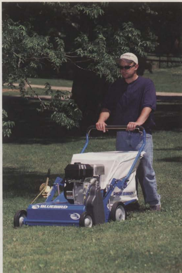
Power raking is a method of dethatching that helps open up a lawn for restoration. Some restoration equipment is available with a bagging option to collect thatch during renovation. Photo: Bluebird
