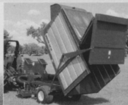
Model BV138 features hydraulic lift unloading
