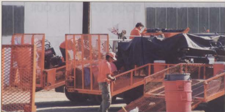
Open trailers can be accessed from both sides and allow contractors to easily reach equipment or load debris from the job.
