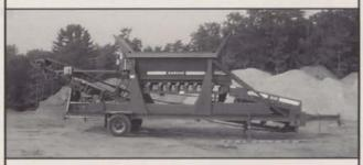
The model 3618 is great for screening topsoil, processed gravel, sand and any other product to meet your needs. Powered by Honda gas engine. Can be fed with a skid steer loader. Very compact for use directly on jobsite. Any size screen opening is available. Quick and easy setup. Features: Remote controlled dumping grizzly, belt feeder, 3' x 6' vibrating screen deck.
