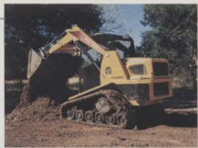
Track loaders' low ground pressure allows them to travel well over both new construction sites and established landscapes. Photo: ASV
