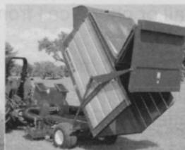
Model BV138 features hydraulic lift unloading
