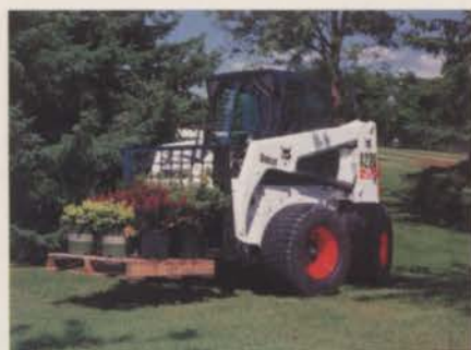
Pallet fork attachments allow contractors to more easily haul plants and other essential materials to their work sites. Photo: Bobcat
