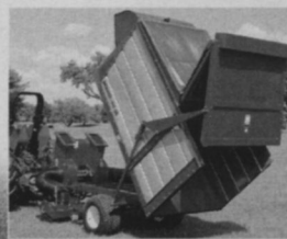
Model BV138 features hydraulic lift unloading
