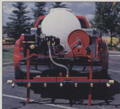
Pickup-mounted liquid deicer application systems are becoming more common.
