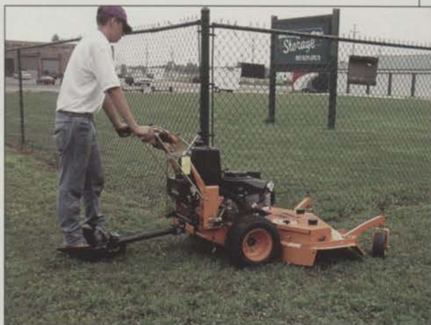
One-wheel trailing sulkies, because of their low weight, work best on gear-drive mowers. Photo: Havener Enterprises
