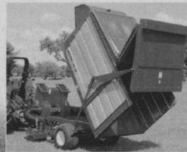
Model BV138 features hydraulic lift unloading
