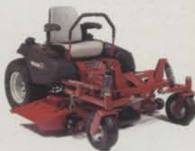
IS® 1000Z. Two-wheel front Independent Suspension for a better ride, smoother cut. 21-HP Kawasaki with 48 inch mower and 23-HP with 52-inch mower.
