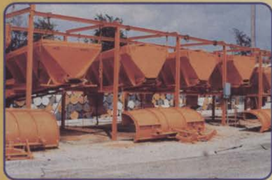
Spreader chains and interior of spreader boxes, tailgate or V-bottom, rust and corrode during off season storage.
