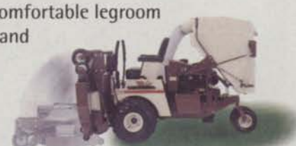
DuraMax™ 90° FlipUp™ Deck (44" to 61"). Bag, mulch or discharge using the same (44" to 72") deck.
