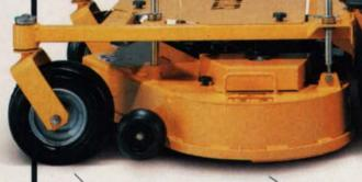
18"x8.00" turf-tread drive tires, the largest on any walk-behind anywhere, for a smoother ride, better flotation, and reduced psi.
