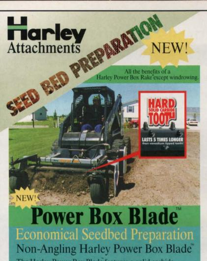
The Harley Power Box Blade features a solid carbide toothed rake fixed in a straight forward operating position
