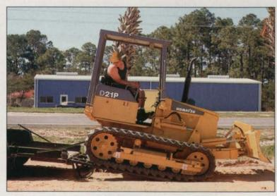
The D21A-7 and D21P-7 compact dozers aren't just smaller, they're lighter. At under 9,250 lbs, they combine unmatched power and controllability with a reliable easy-to-transport design. From durable all rubber tracks, to single lever 6-way PAT blades, these versatile dozers are perfect for landscapers who demand reliability and ease-of-use.
