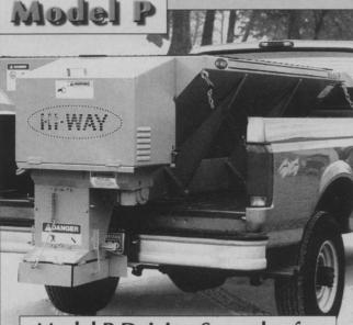
Model P Deicing Spreader for winter salt and sand application
