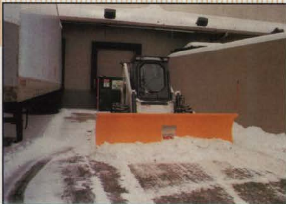
Snowplows are available in plastic and steel. The plastic blades, although lighter in weight, are not as strong as their steel counterparts and may require additional bracing. Photo: Snow Wolf
