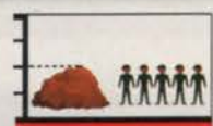
5 MEN AND A WHEELBARROW A typical 5-person crew can spread 8 cubic yards per hour.
