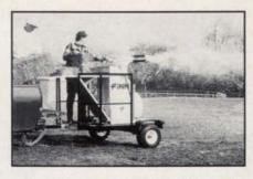
· Straw blower is powered by a 20-hp Kohler engine
