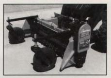
GLENMAC HARLEY POWER BOX BLADE • Non-angling for skid-steer loaders • Features a solid carbide-toothed rake that is fixed in a straight forward operating position (continued on page 158)
