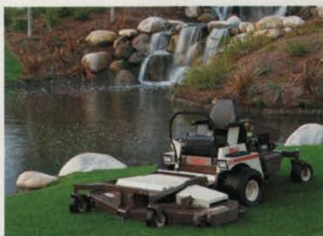
28 hp 928D 2 with heavy-duty 72-inch deck.
