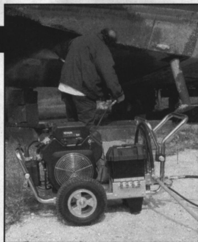
The first thing contractors look at when purchasing engines is horsepower, followed by the choices between twin-cycle or single-cycle, liquid-cooled or air-cooled and overhead-valve or side-valve engines. Photo: Kohler
