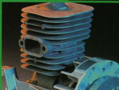
Chrome-plated cylinder for longer life.
