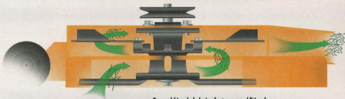
One mulching deck design features an additional, upper deck located above the middle blade of the mower to hold the grass clippings above the bottom cutting deck longer, giving it another chance to run through the three blades.
