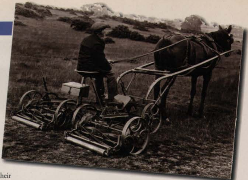
(Above) An example of a side-wheel gang mower. Photo: Textron Turfcare & Specialty Products (Lower left) Hustler's 1964 zero-turn riding unit with a belt drive and lever steering. Photo: Excel Industries
