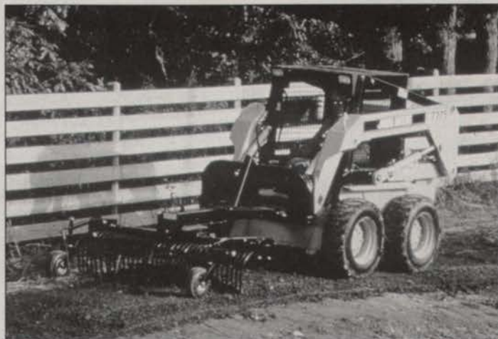
Contractors demands for maximum versatility from skid steers forced manufacturers to adapt a universal attachment system so attachment tools work with a variety of skid steer machines. Photo: Deere & Co.
