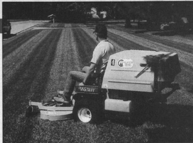
Riding mowers are particularly popular on larger projects that don't require a great deal of tight turning. Photo: Walker Mfg.
