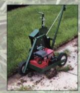
Edge-R-Rite by Turfco Mfg. Quit using the Edge-R-Rite by Turfco Mfg. Quit using shovels and trenchers to edge flower and bush beds; the Edge-R-Rite does it quickly and cleanly. The five unique blades also make installing all kinds of edging easy and profitable. Concrete or brick tree rings can be installed in minutes. Save hours of labor on edging and installations, wire installation, drainage problems and general edging. A power shovel does sidewalks too! Circle 622 on reader service card
