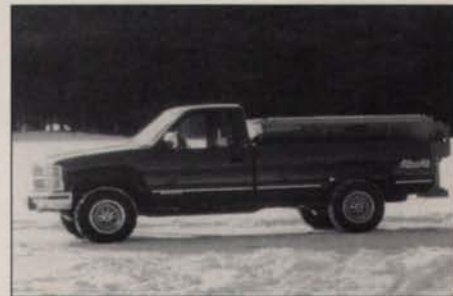
Check all of the wiring, cable connections and bolts, as well as the spreader itself, before using each winter. Credit: Highway Equipment
