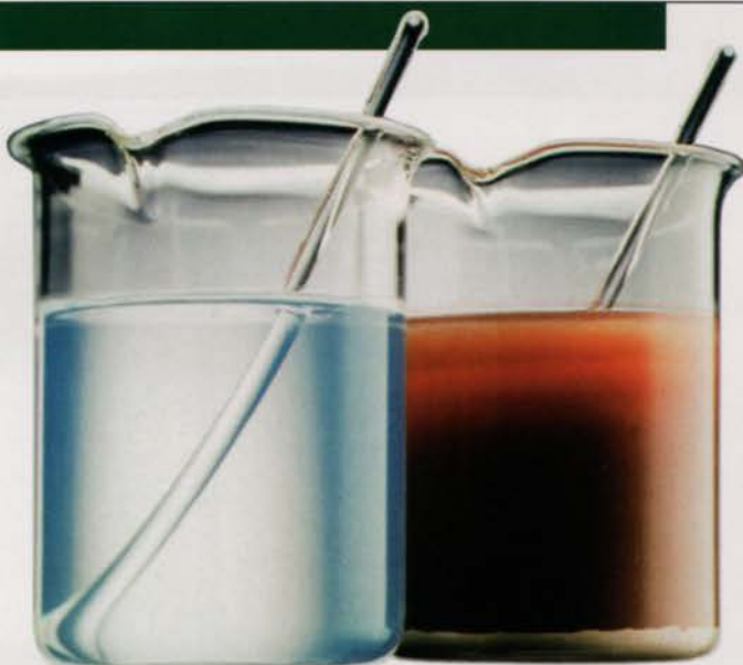
Banner MAXX (left) is a water-based fungicide that forms an ultra stable suspension, unlike powders (right) or emulsifiable concentrates, and is widely compatible in a tank mix.
