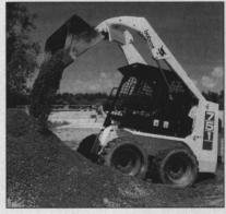
model comes with a unique cooling system that brings cool, debris-free air in from above and through the radiator and oil cooler before mixing it with engine air and exhausting it out side vents. This design is said to help keep engine components clean.
