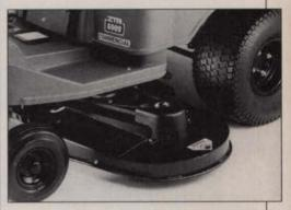
radius and a durable body that tilts up for easy servicing. Deck widths range from 30 to 60 inches.
