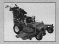
wet conditions. The Quick-Lift cutting height adjustment eases going over curbs and loading into trailers, and the HydroTrac tracking adjustment aids straight tracking on slopes and other conditions. Units are available with 36-, 48-, 52- and 61-inch deck sizes, and offer four Kohler engine options ranging from 16- to 20-hp.
