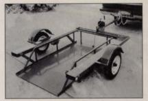
Ground level loading trailer from **Premco Products** eliminates simple loading problems typical of ramps or tilt trailers. The Triple L trailer attaches to a tow vehicle to provide a deck that can be lowered flat to the ground. Slide equipment into position and use a self-locking winch to raise the load into travel position. Features include independent suspension,
