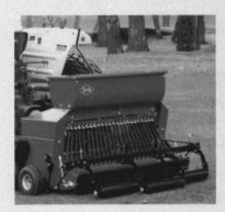
Our 48"-wide unit creates 24 separate slits on 2" centers. Cutter blades are heat-treated spring steel with sawtooth design. Precise metering 24 seed tube outlets assure even seed distribution and placement. You get faster, thicker turf growth.
