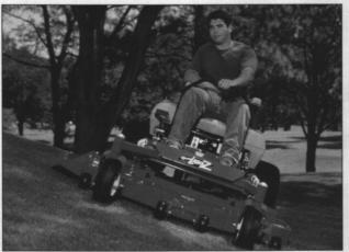
Hillside mowing is a learned art and operators should be taught how to handle the mower to reduce the chance of losing balance.
