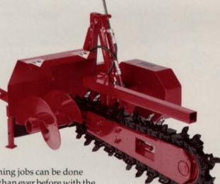
Trenching jobs can be done faster than ever before with the Steiner TH300 Trencher. Mounted quickly to the front of any Steiner 4wd tractor, the TH300 tracks precisely down the line of trench, cutting to a maximum depth of 28". A highly visible depth indicator and variable depth control gives you complete control over the heat treated, carbide tip trencher.
